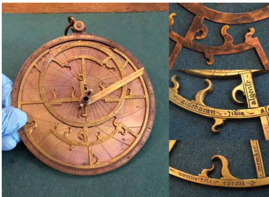
Fig. 5 Fusoris-style astrolabe in the University Museum of Utrecht, inv. um.342 (left), front view and (right) details of front and back of rete showing workmanship. Courtesy of the Universiteitsmuseum Utrecht (photos Kenneth Launie).
