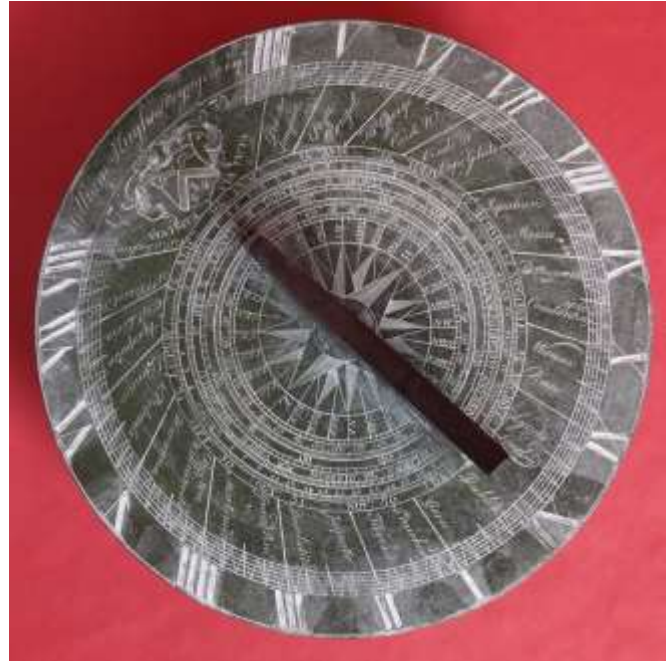
Fig. 2. Plan view of the dial, dusted in talc to emphasize the engraving.
