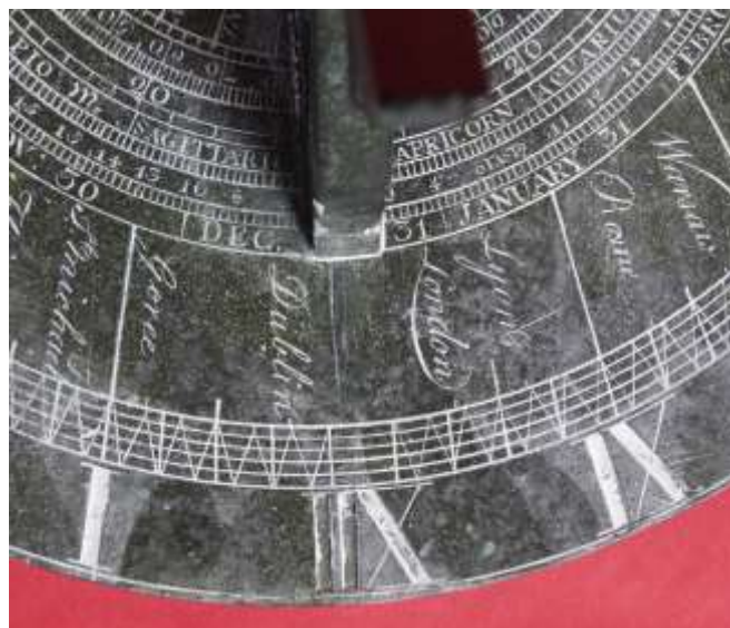
Fig. 8. Close-up of the dial-plate showing the transversals and the geographic place-names.
