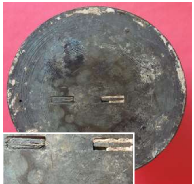
Fig. 6. The back of the dial. Inset: a close-up of the gnomon tenons and the name "Owen".
