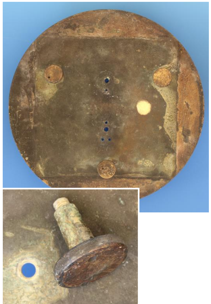
Fig. 6. Back of the Gabriel Davis dial, showing the three 'mushroom' fixings with tapered shafts. Inset: the 'one-dot' pedestal fixing. The marks in the patina show that at one time the dial was mounted on a square capital. The shiny spot is the area cleaned for XRF.
