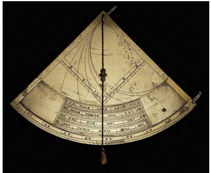
Fig. 3. The British Museum quadrans vetus , an unequal-hour quadrant with moving cursor. Courtesy of the Trustees of the British Museum, inv. no. 1972,0104.1.
