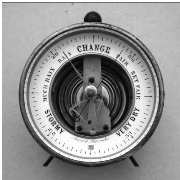
Fig. 1 Aneroid barometer (70mm in diameter).
