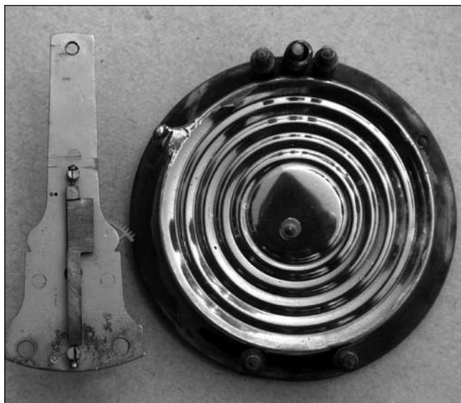
Fig. 3 Close-up of capsule with point and the lever.
